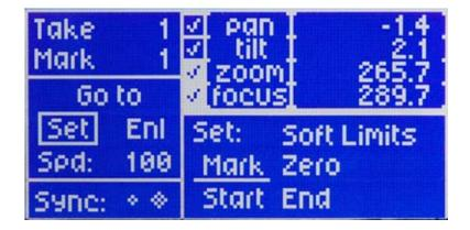
Mark: Sets the current position of all motors in internal memory. Assigns the mark number on the screen to refer to this position.
