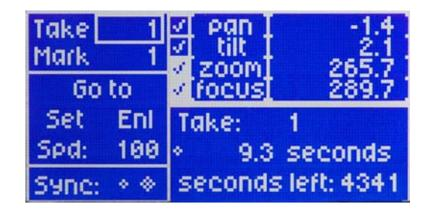
2) Mark - Marks are pre-recorded positions for pan, tilt, zoom and focus. This control shows the selected Mark number. You can select up to 2000 pre-recorded positions. As this number is changed, the motor positions for the selected mark will show on the screen. After selecting a new take or mark, press "Accept" to keep the new number, or "Cancel" to revert to the old value.
