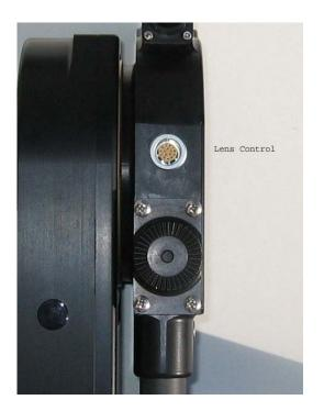
The Talon lens control system is incorporated into a small circuit board located in the tilt box. A single 16 pin LEMO connector brings all lens controls to the outside. These controls include:
